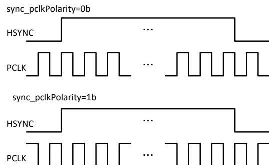
**Figure 9 PCLK polarity**
