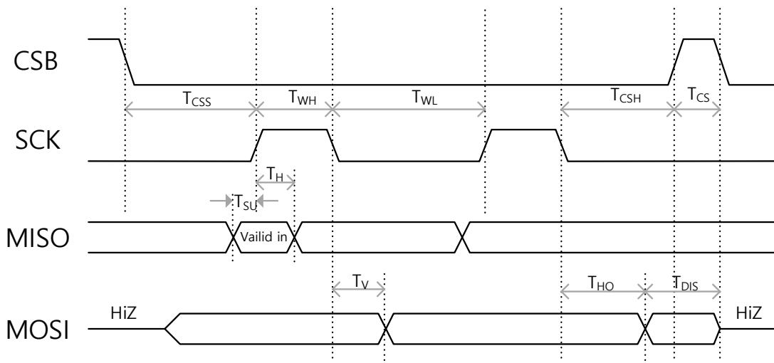
**Figure 46 SPI timing diagram**
