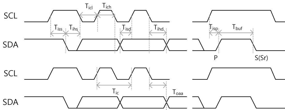
**Figure 45 Timing diagram of SCL and SDA**
