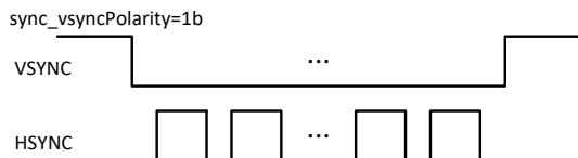
**Figure 7 Vsync polarity**
