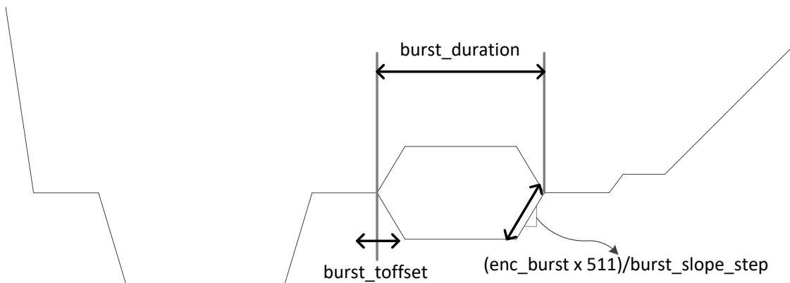
**Figure 41** Burst timing
