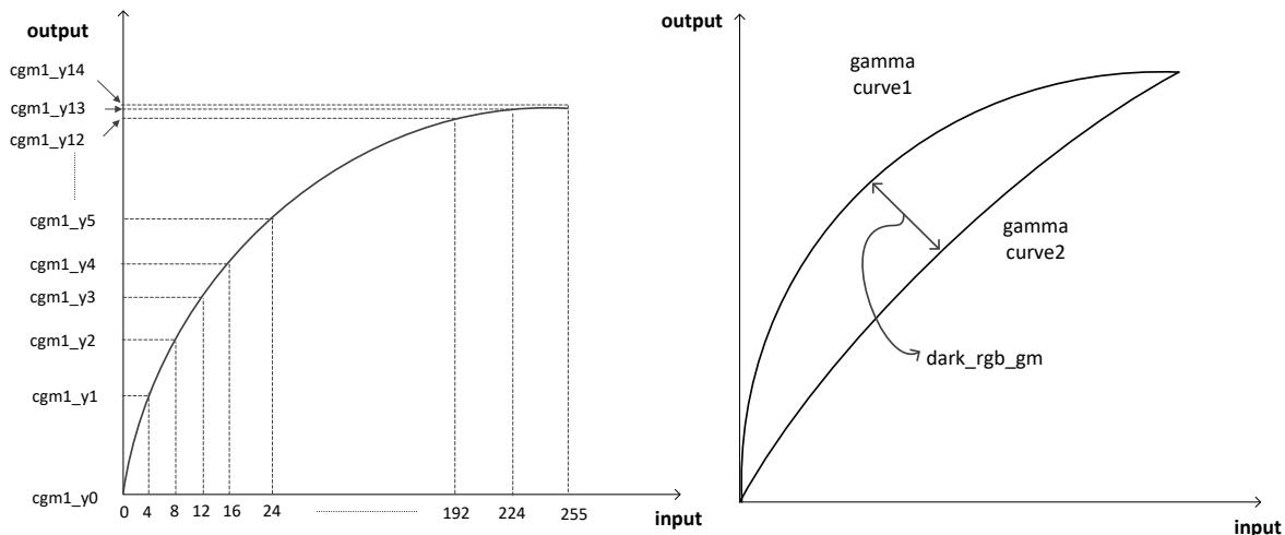
**Figure 33 Gamma curve fitting of RGB gamma**
