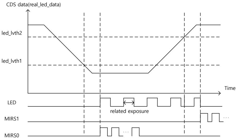
**Figure 23 LED control with CdS**
