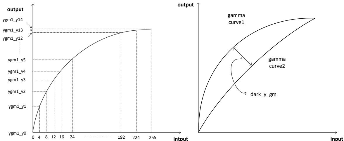
**Figure 34 Gamma curve fitting of Y gamma**
