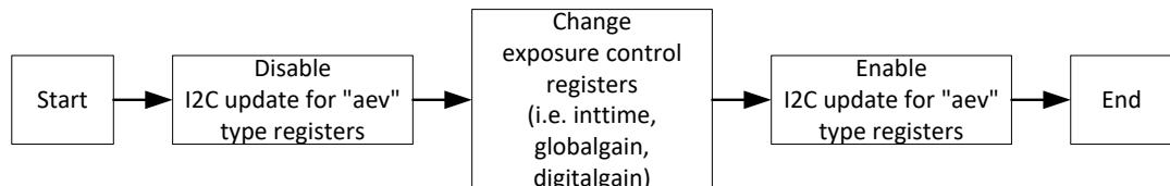
**Figure 27 Recommended exposure setting sequence**
