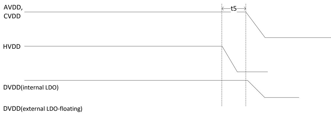
**Figure 15 Recommended power down sequence**
