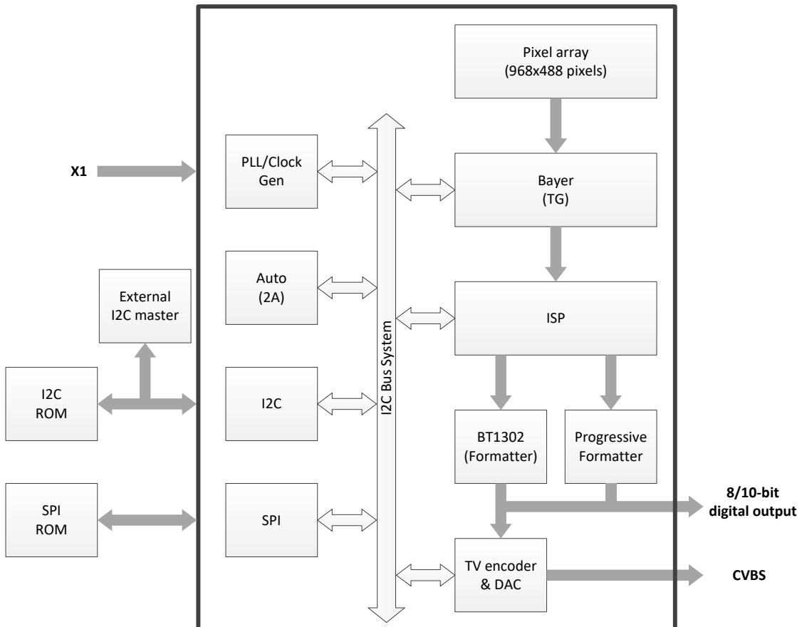
**Figure 1** Chip architecture
