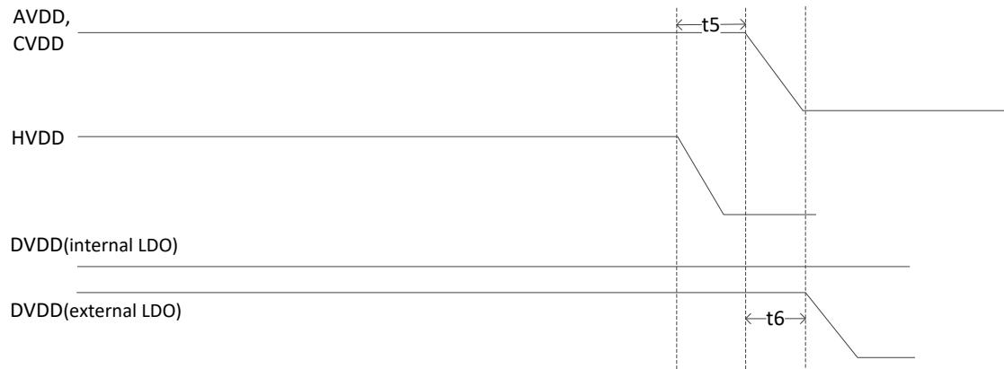
**Power-down Sequence(using internal LDO)**
