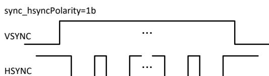
**Figure 8 Hsync polarity**
