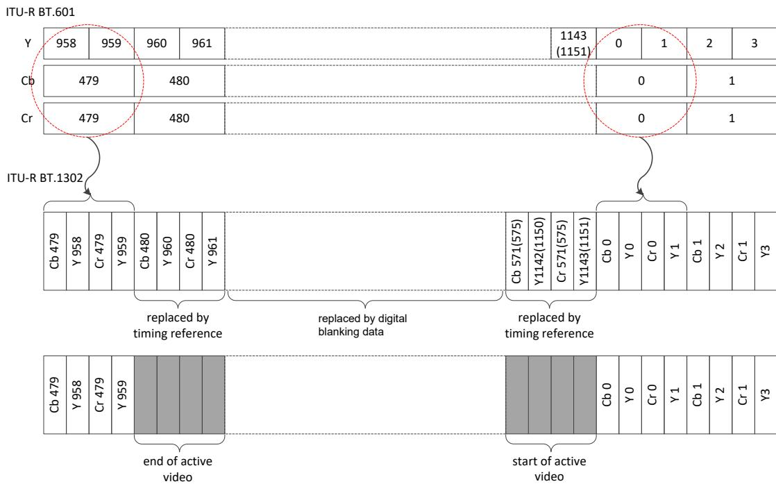
**Figure 11 Timing diagram for ITU-R BT1302**
