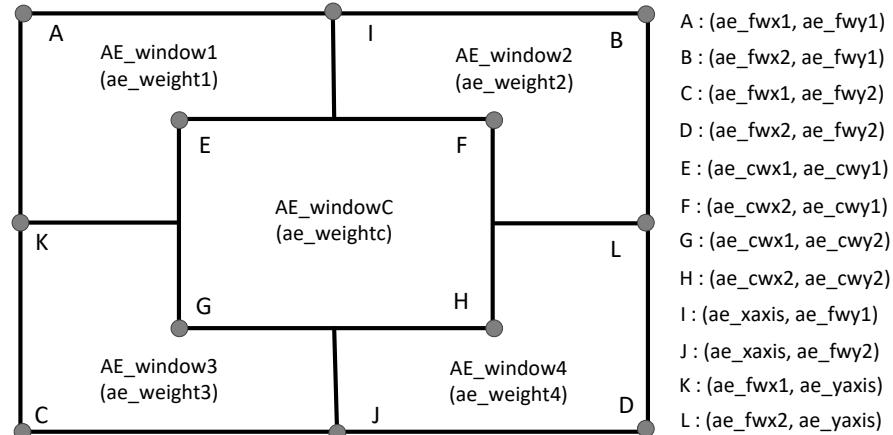
**Figure 38 AE window setting**
