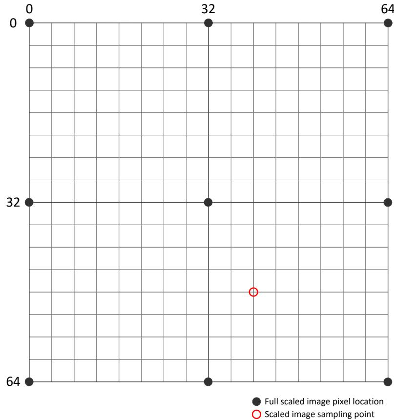
**Figure 10 Example of scale down**
