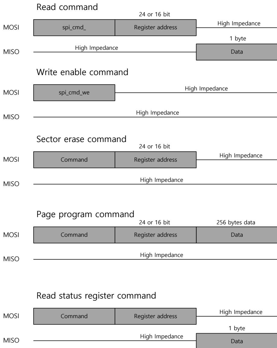
**Figure 22 SPI functional description**
