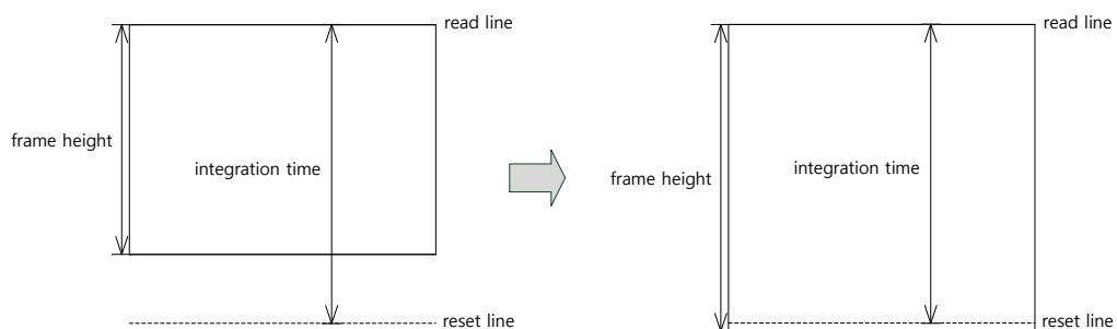
**Figure 25 Integration time with frame variable mode enabled**
